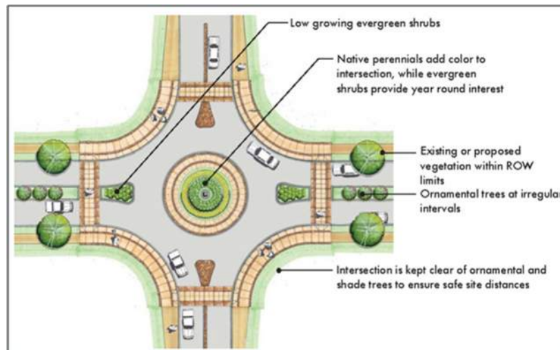
Example Enhanced Pedestrian Crossings at Roundabout:
